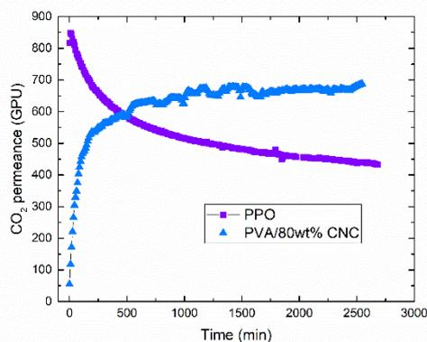
**Figure 2.** Comparison of long-term separation performances of PPO support and PVA/CNC composite membrane
