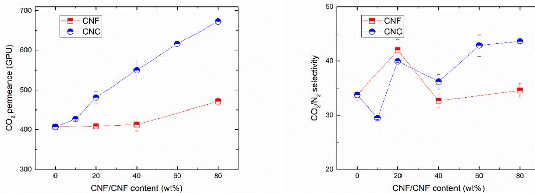
Figure 1. CO<sub>2</sub> permeance (left) and CO<sub>2</sub>/N<sub>2</sub> selectivity (right) of PVA/CNC and PVA/CNF with different additive content at 100% RH.
